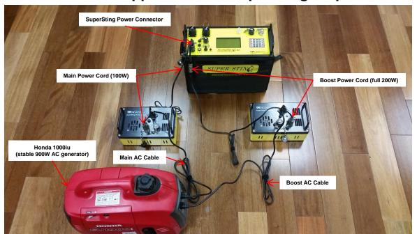
For project planning, the SuperSting Generator Power supplies require a 900W generator. The Honda 1000iu is a popular choice. This generator needs to be ungrounded (optional and seldom used). Make sure nothing else is plugged into the generator. The SuperSting will then be isolated from ground loops.
